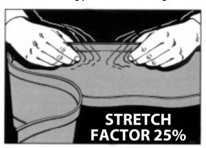
The edges of Dekstrip® contain an expanding aluminium strip (in concertina form) totally encased by the E.P.D.M. rubber flashing. The strip allows the flashing to be stretched and formed around most roof profiles - and maintain that shape. Fastening may be done through the aluminium strip using fasteners with a minimum
