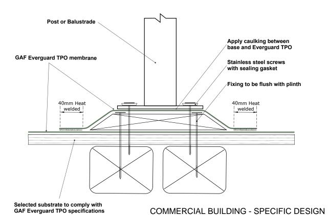
DRAWING: DATE: DETAIL: POST OR BALUSTRADE BASE 407 6 DEC 2019 **DETAILS FOR:** SCALE: N/A **BRANZ Appraised EVERGUARD TPO ROOFING** Apprasal No 529
