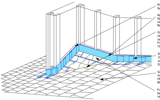
Provide continuous support to flashing upstand
