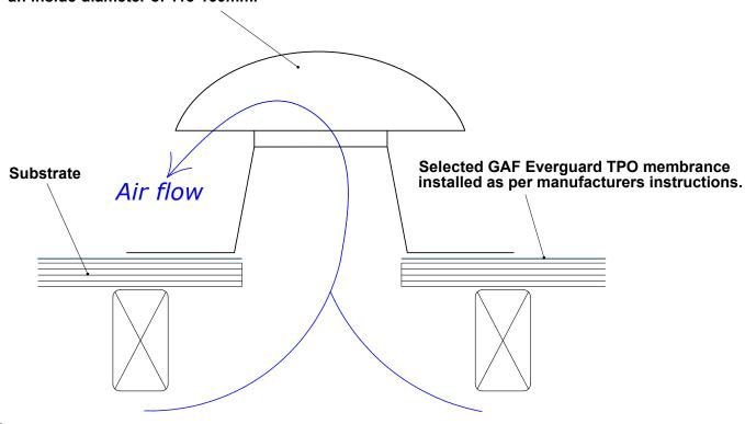
1. Use 2 GAF Masterflow vents per 70m2 area. Ensure cross flow ventilation between blocking supports. 2 Castellated battens can be used under plywood substrate or 20mm holes applied to the blocking. 3. Substrate to comply with GAF substrate checklist readiness sheet www.gafroofing.co.nz/tpo-docs/
