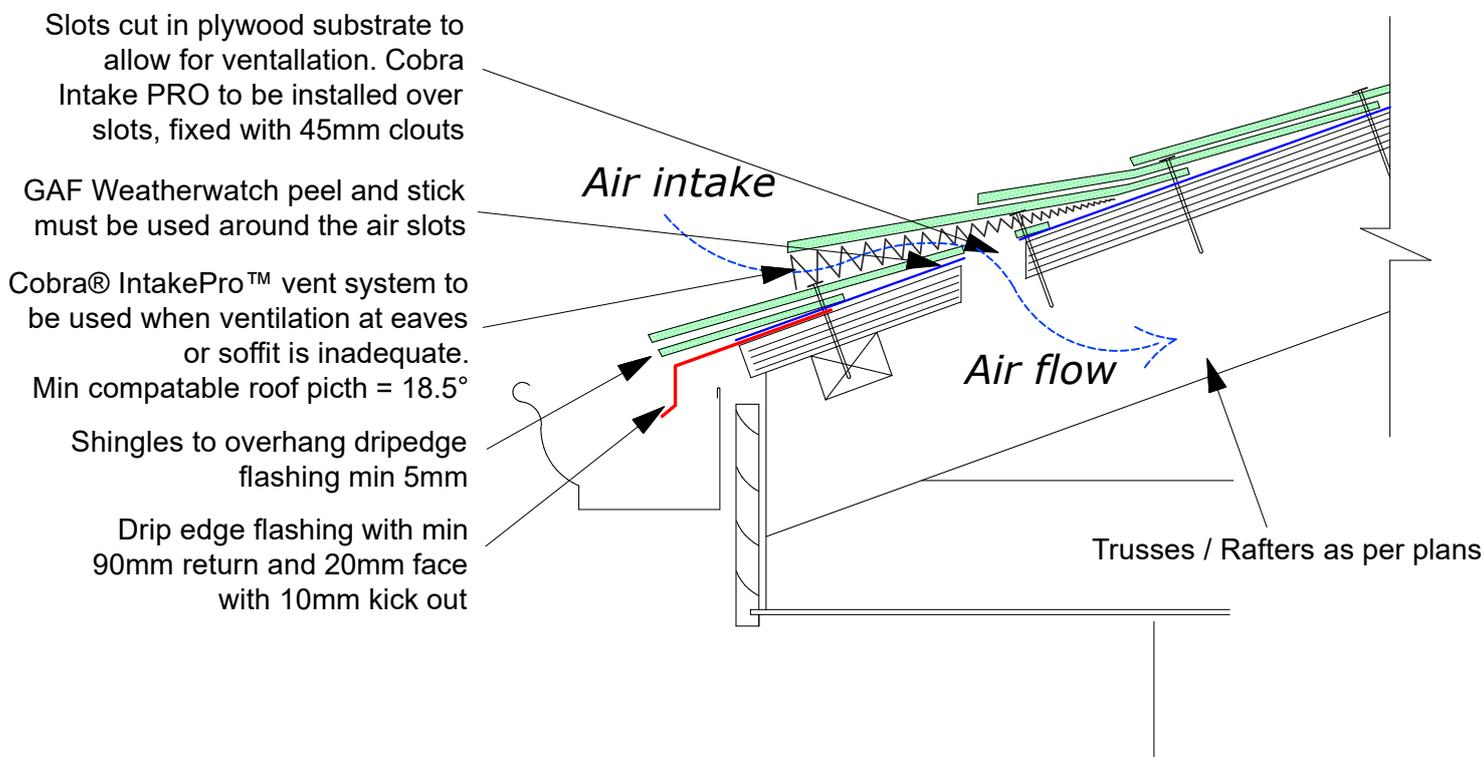
Slots cut in plywood substrate to allow for ventilation. Cobra Intake PRO to be installed over slots, fixed with 45mm clouts
