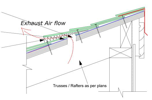
Slots cut in plywood substrate to allow for ventallation. Cobra Intake PRO to be installed over slots, fixed with 45mm clouts
